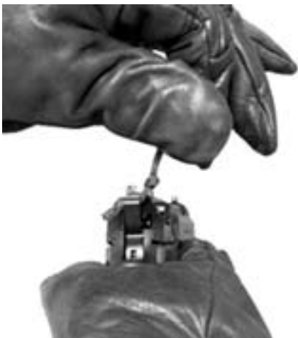
Figure 1-22. Cocking the Pistol with 550 Cord.
